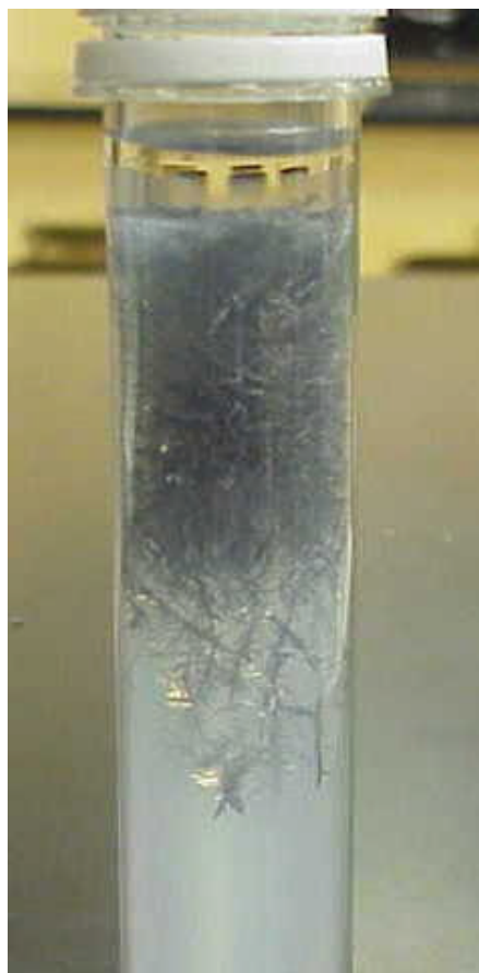
\text{Pb(NO}_3)_2 in gel, Zn(s) stuck into surface. \text{Pb(s)} forms.
