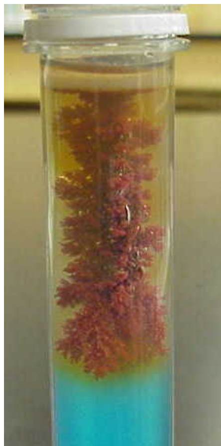
\text{CuSO}_4 in gel, Fe (paperclip) stuck into surface. \text{Cu(s)} forms.
