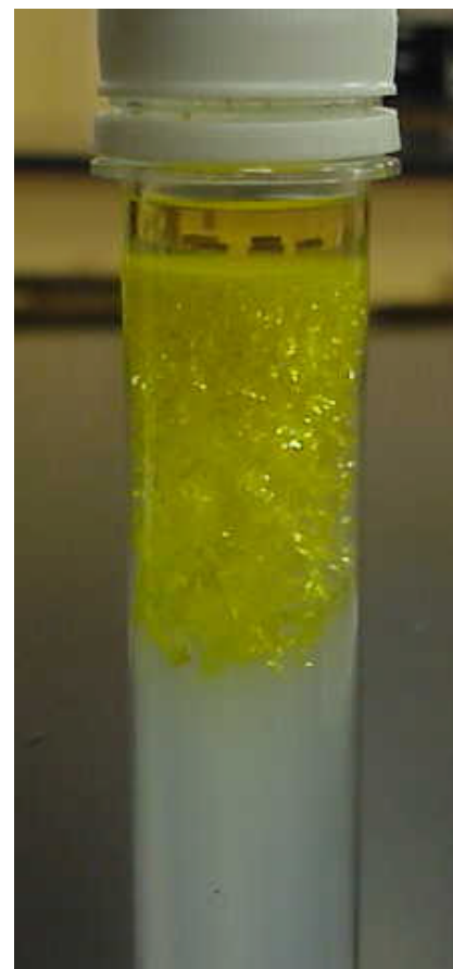
\text{Pb(NO}_3)_2 in gel, KI(aq) floated on top. \text{PbI}_2(\text{s}) forms.
